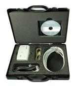
The OCI700.1 service tool (see Data Sheet N5655) consists of a service case containing a CD-ROM with the ACS790 software, the OCI700 service interface and 3 device-specific connecting cables.
