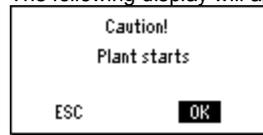
10. Press the select-and-push knob for OK. The application will be started, all sensors will be checked, and sensors used will be highlighted for error messages that may be required later. The main menu will appear:
